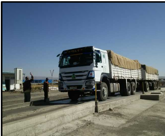
Axle Load Control facility
